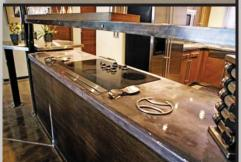
This loft kitchen has custom bamboo wood doors paired with the grain turned to 45 degrees, mixed with a pattern of custom welded stainless steel drawer fronts and doors, layered with glass. The stainless steel backsplash flows into the concrete countertops, which match the finish of the floor. The cabinets are topped off with a bulky wood bamboo valance, intertwined with blackened steel I beams, which continues the theme as a steel angle suspends the open shelf over the cook top.
